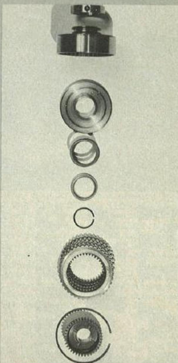
A disassembled clutch reveals all of the internal working parts. From top to bottom they are the hub's bearing/collar, the clutch hub, piston, piston return spring, retaining collar, snap ring, clutch plates, the gear and drive hub and the plate-retaining snap ring.
