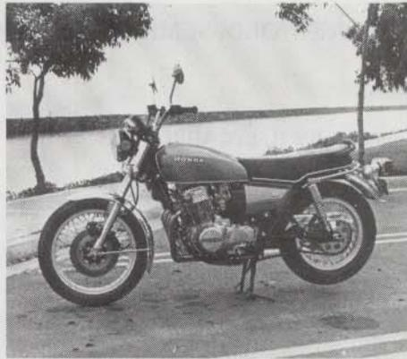
A full fuel tank runs the Honda's weight to approximately 590 pounds, qualifying it as a legitimate heavyweight. Wheelbase is 58.3 inches, seat height stands at 32.3 inches. The combination of disc brake on the front, internal expanding shoe on the rear is an excellent choice for touring. The front tire is a 3.50 X 19, the rear tire is a 4.50 X 17. Alloy rims and semi-valanced front fender are features first introduced on the GL 1000.
