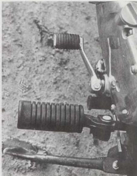
The gear selector is still around, even though its function has been diminished to semi-retirement. "Shifting" pattern is down for neutral, up for Low Range, up again for Drive. The sidestand automatically returns the transmission to neutral when deployed.
