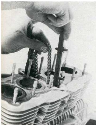
**23.** The adjusting screw and the top bolt that retain the cam chain tensioner were removed earlier. The tensioner must be rotated 90 degrees so its integral guide pins will clear the chain slot in the cylinders and it can be lifted from the cylinder barrel. The chain stays for now.
