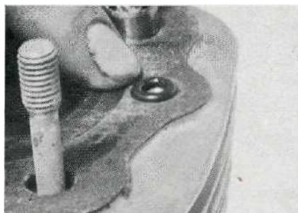
**24.** There are several rubber O-rings and aligning pins in both the cylinder head and barrel (another reason for having the factory workshop manual handy). Remove these oil passage O-rings from the cylinder barrel, for example, so you don't lose them. Remember to replace them!
