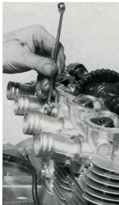
13. The bolt immediately above the cam chain tensioner is the one that actually holds the tensioner in the cylinder head. You must remove it to remove the cylinder head. Leave the actual tensioner in place for now (it can stay in place if you're only working on the head).
