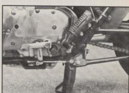
This separate shift linkage pops the gearbox into neutral when the sidestand is extended, and prevents the engagement of any gear until the stand is retracted.
