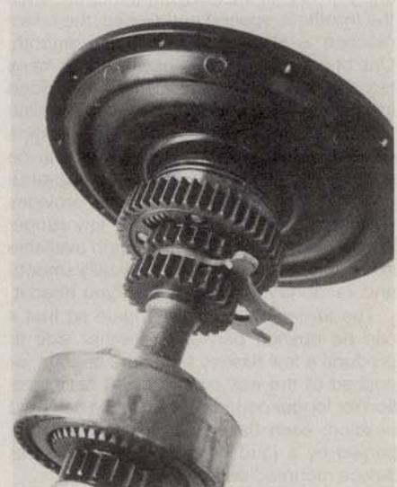
Gearbox mainshaft shows detail on shifting clutch, stator reaction arm, and sprung converter gear.
