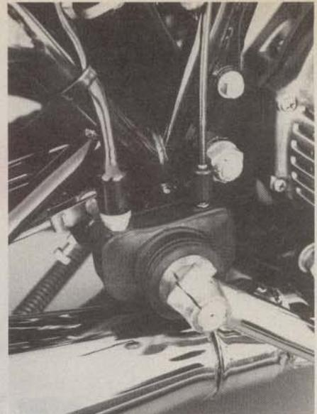
Rubber boot on rear brake lever pivot covers stop switch and cable-controlled ratchet on park brake.
