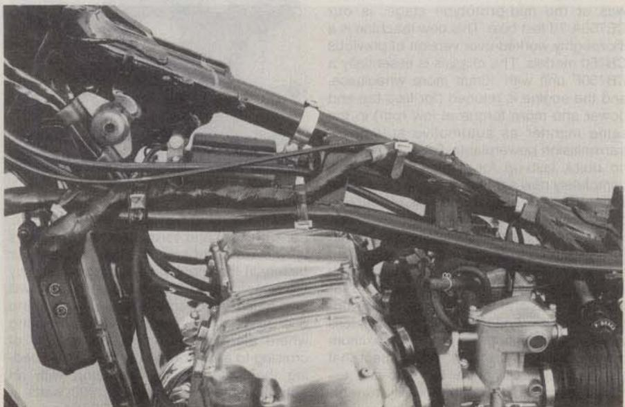
Plastic box on frame downtube holds the wiring connectors so electrical problems can be found fast.
